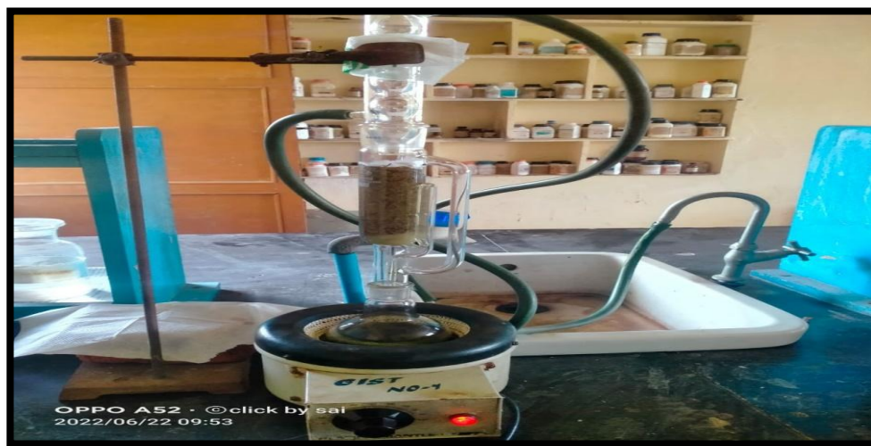
Figure : 4 Psidium guajava leaves extraction by soxhlet apparatus.
