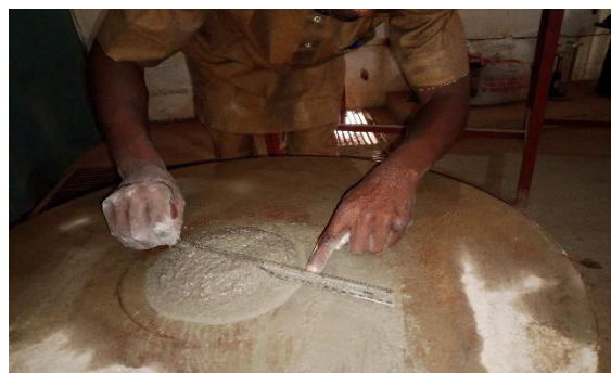
Plate IIc. (Plate II a-c Showing the flowability test of the mortar produced).
