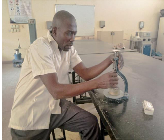
Plate III; Setting time of mortar
