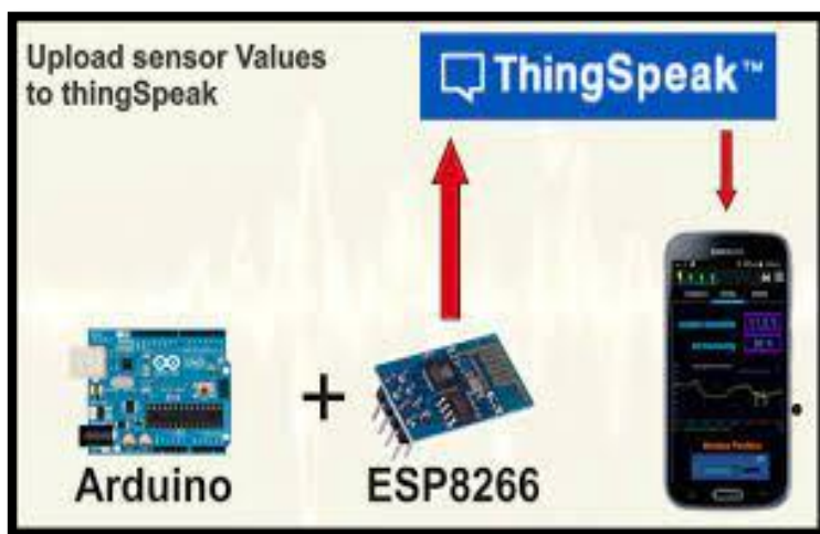
Fig5: Data Transfer using ESP8266 to Things peak application
