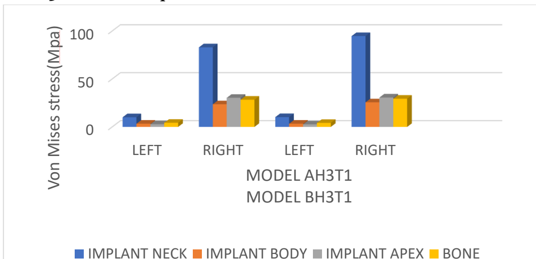
Graph 10- Comparison of von Mises stress values in different regions of model AH 3 T 1 , BH 3 T 1 under vertical load
