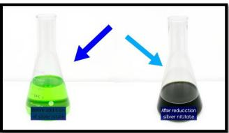
The observed color shifting due to the surface plasmon resonance (SPR) of the silver nanoparticles, pointed out the existence of their creation.
