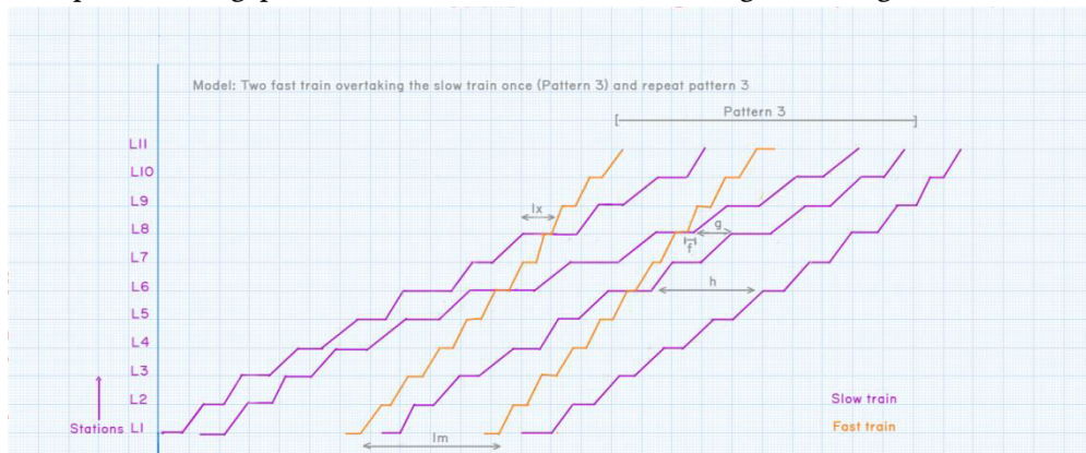
Fig. 6 Two fast train overtaking the slow train once and repeat this pattern
