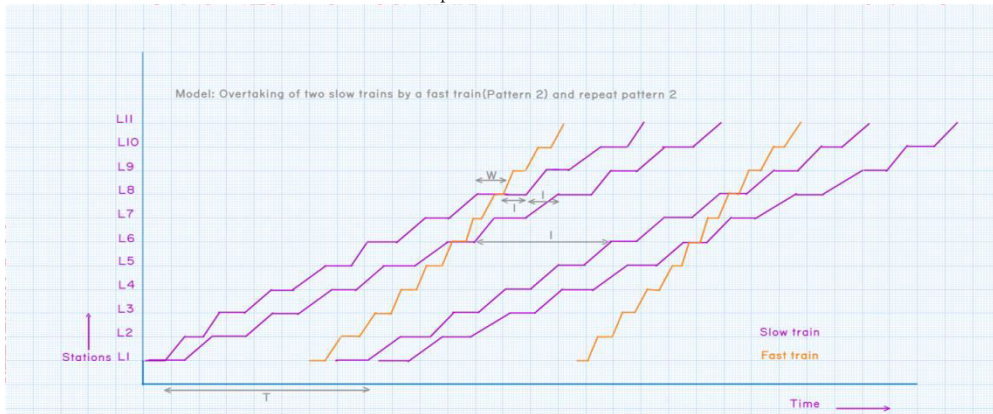
Fig. 4 Overtaking of two slow trains by fast trains and repeat this pattern
