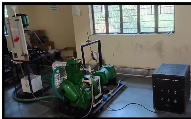
Figure-3: Single-cylinder, four-stroke diesel engine setup
