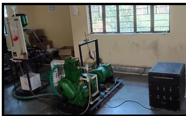
Figure-3: Single-cylinder, four-stroke diesel engine setup
