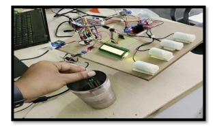
A water backflow prevention device managesflooding using key components. It features a NodeMCU Microcontroller for remote monitoring and control via Wi-Fi. Moisture Sensors detect water levels, sending alerts to the Node MCU when thresholds are exceeded. The device also includes H-Bridge Motor Drivers, Suction Motors, and Servo Motors to pump out water and manage barriers. These components work together to prevent flooding and restrict vehicle access to affected areas.
