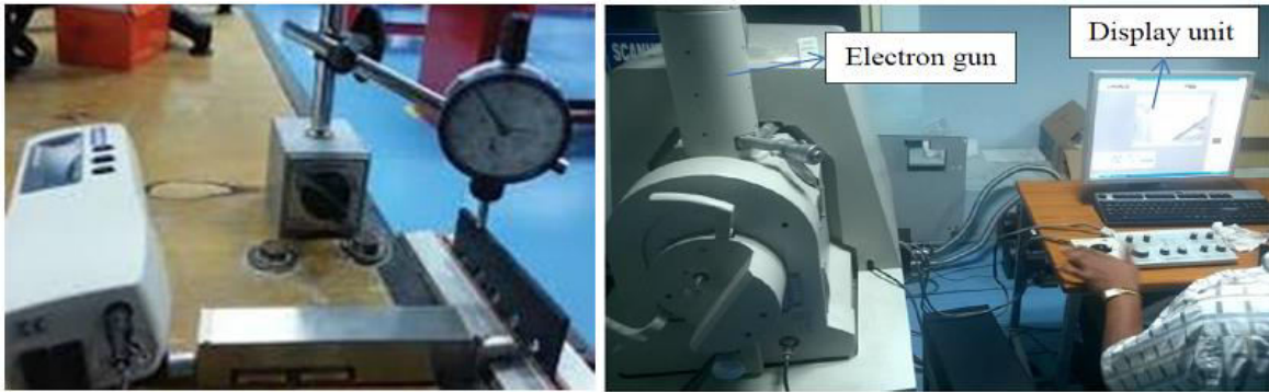
Fig 2 and 3: Surface roughness tester and SEM used to measure flank wear of drill tools
