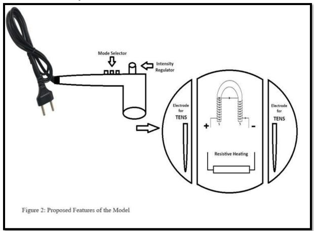
Components: The proposed model consists of three main components: a heating element for SHM, a PEMF generator, and electrodes for TENS. These components are integrated into a single device controlled by a microcontroller unit (MCU). The MCU is connected to a remote control interface, allowing healthcare professionals to adjust therapy parameters such as intensity, duration, and mode of operation.
