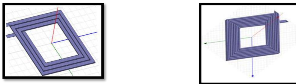
Fig.6.(a) Structure of ML Constant width Inductor b) Structure of ML double Split Inductor
