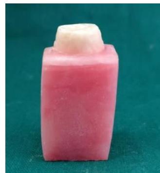
Fig. 2: Creation of Space Cavity of 5 mm in length, 2 mm in depth
