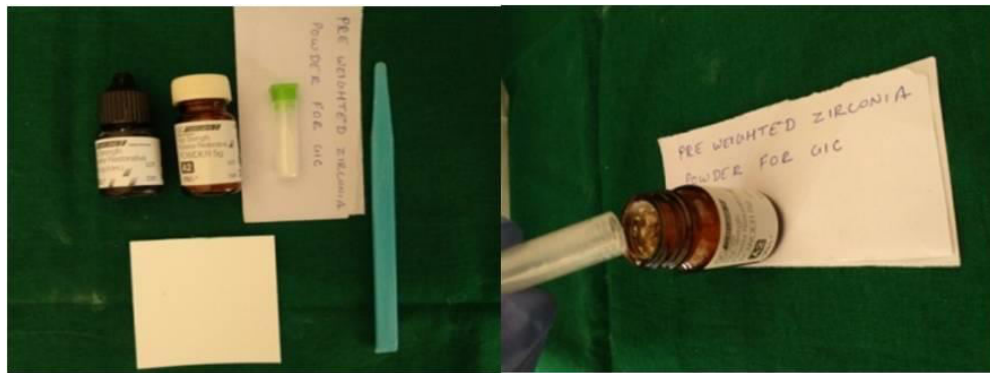
Fig. 3: Pre-Weighed 10% Zirconia powder added to GIC Powder
