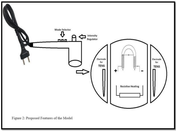
**Components:** The proposed model consists of three main components: a heating element for SHM, a PEMF generator, and electrodes for TENS. These components are integrated into a single device controlled by a microcontroller unit (MCU). The MCU is
